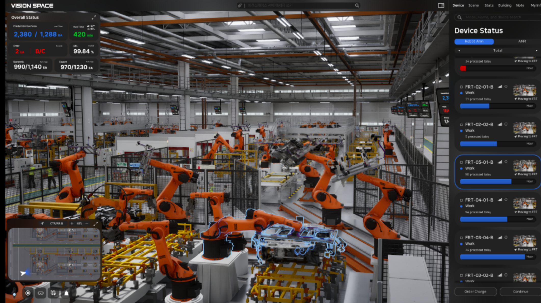
Simulation and Monitoring for H Client's EV Body Plant - 14,000 square meters, 96 robots integrated
