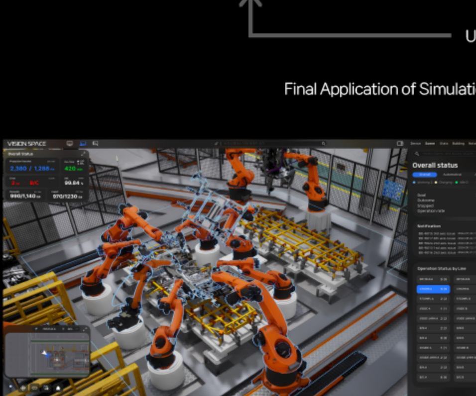
Real-time Monitoring of automated production processes [Predictive maintenance based on robot, protocol data linkage possible]
